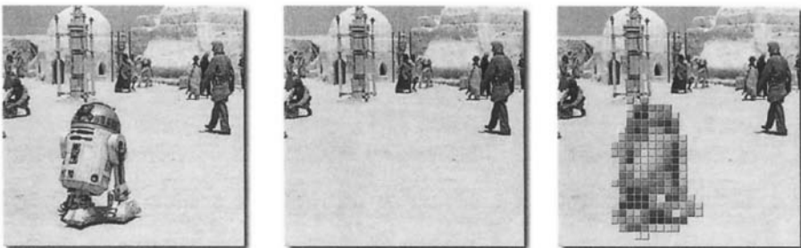
Figure 10.3. Original image, tampered image, and detection of tampered regions. (Courtesy of D. Kirovski's Power Point presentation).
