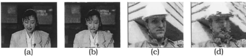
Figure 6.9. Images (a) and (c) show the original MPEG frames from "Akiyo" and "Foreman", respectively. Images (b) and (d) show the visual defects caused by encrypting the sign bits of motion vectors in low-motion sequence "Akiyo" and high-motion sequence "Foreman", respectively.
